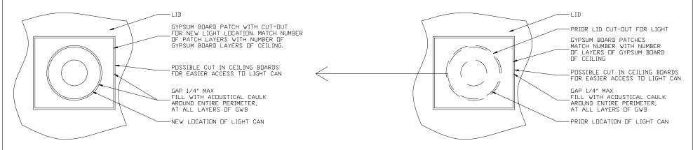
ALSO APPLY RECESSED LIGHT BOX-DUT DETAIL AT NEW LOCATION. SEE DETAILS VD-1A AND VD-1B AS NEEDED -SECTION AND BOTTOM VIEWS.
